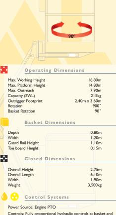
Controls: Fully proportional hydraulic controls at basket and ground.
